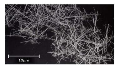
Average Fiber Length: 15 µm Average Fiber Diameter: 0.5 µm
